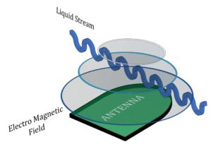
emits a narrowband EMF into the liquid. The system sweeps through a frequency range creating a spectrum of the liquid's EM-response and calculates specific features from the spectrum in real-time. The generated EMF is a directional and short-range field. The used frequencies and emitted energy are harmless, like signals in standard telecommunication systems like mobile phones.
